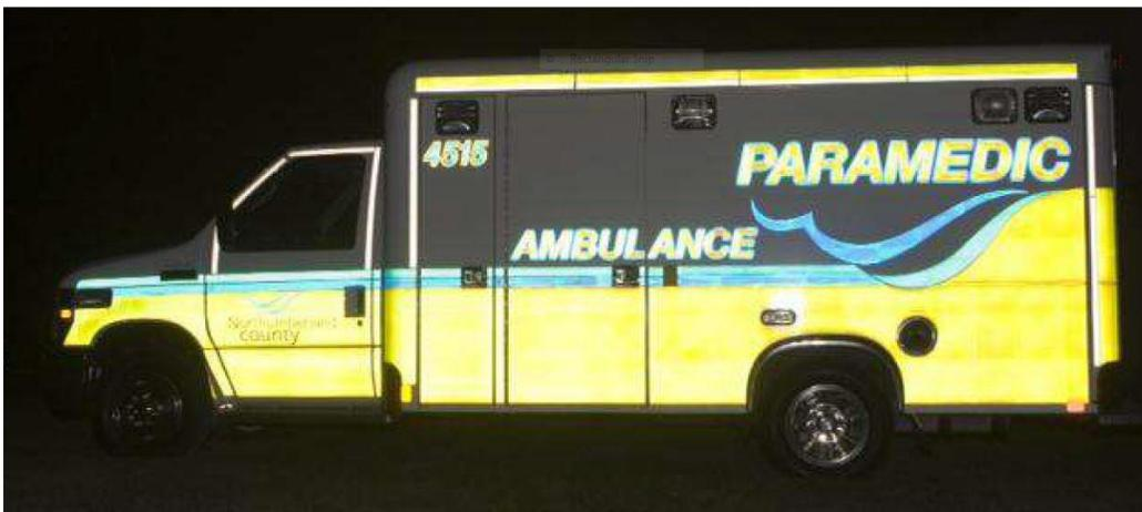
The difference above is quite noticeable. On the high visibility ambulance, a reflective white stripe outlines the cab and body showing the size and shape of the vehicle. The high visibility green at the top of the box outlines the vehicle and adds to side visibility, especially during traffic movement. Large block lettering allows the vehicle to be easily identified. As per requirement of the Ambulance Act, the lettering is also highly contrasted.
